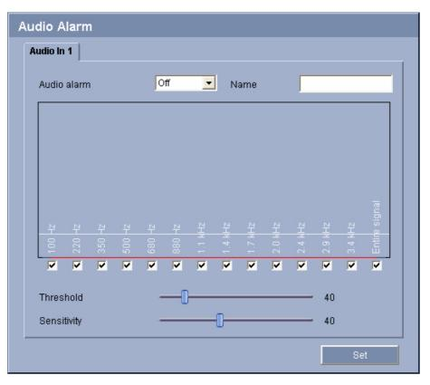
The VideoJet X10 SN can create alarms on the basis of audio signals. You can configure signal strengths and frequency ranges in such a way that false alarms, for example due to machine noise or background noise, are avoided.
